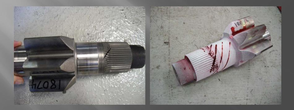
Steering sector shaft failed on previous slide. Investigation of this accident concluded *failed* <u>steering sector shaft!</u>
